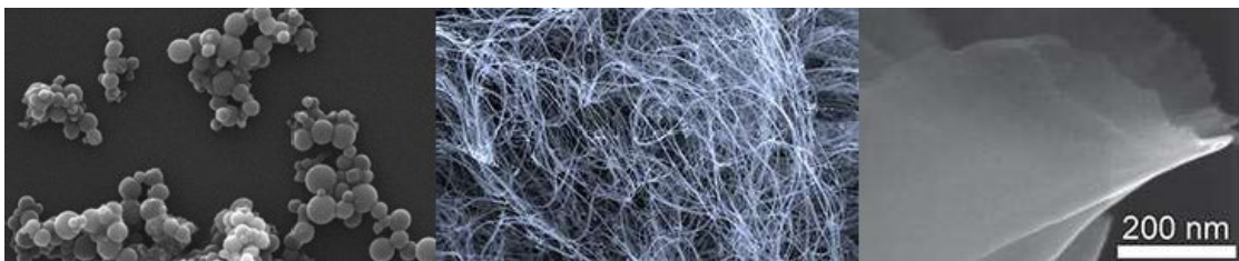
Welding smoke particles; carbon nanotubes; titanium dioxide nanocoatings (source: BauA)
